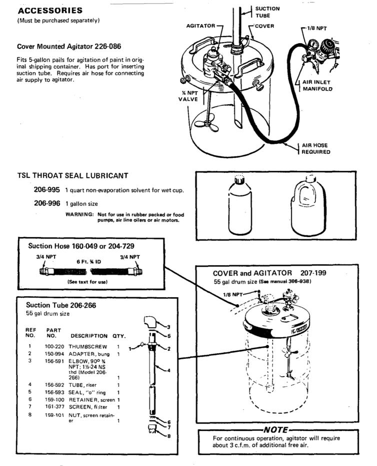
For agitation of paint and suction directly from original 55-gallon shipping container. 6-ft. suction hose 160-049 is for petroleum base solvent flushing and water base materials: 204-729 is for hydracarbon solvent flushing materials.
